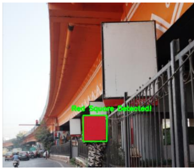
Fig 3: The original image of the red board being processed and hence the red board being detected.
