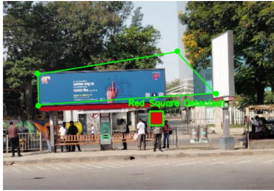
Fig 4: Draggable points being positioned at the corners of the hoarding, with the detected red reference box visible in the image near the hoarding.
